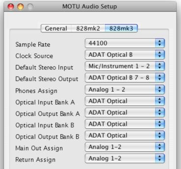
b) For the 828mk2, set both the Optical Input and Optical Output to ADAT. Set the Clock Source to ADAT Optical.
